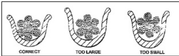
Fig 7-2-1 Correct and incorrect sheaves for a rope
